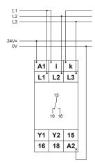
Connected to 1~ 230V mains with power module 230V AC without fault latch  $\rm I_{N}{<}12A$
